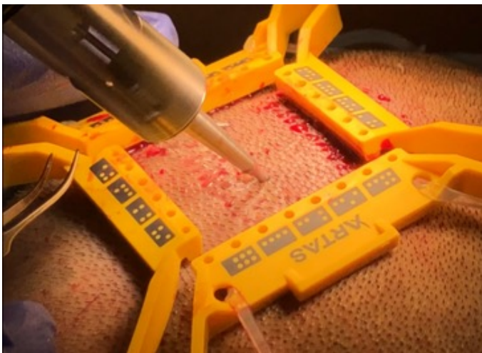
Fig. 2 a) ARTAS iX excising an individual follicular unit. b) ARTAS iX creating a recipient site and inserting a graft from a loaded cartridge.
